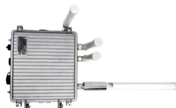
LoRawan outdoor base station
